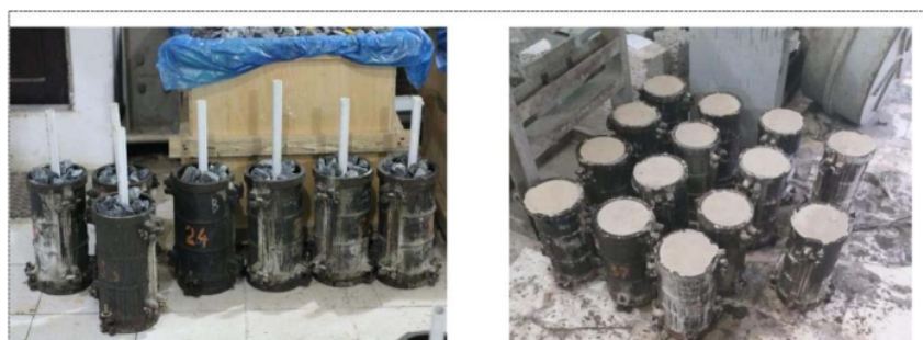
Figure 6. PAC Specimens in Laboratory
