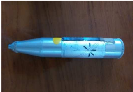
Gambar 1. Schmidt hammer test
