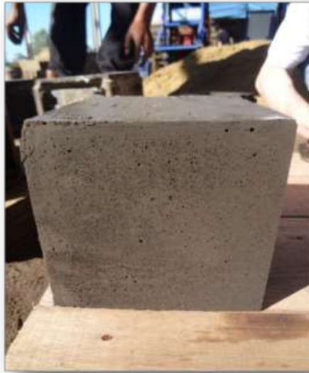
Figure 1 Lightweight brick under study
