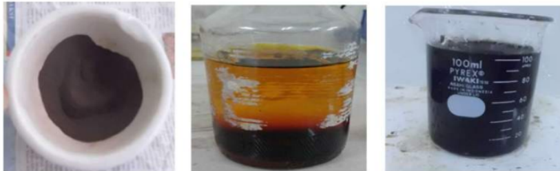
Figure 1. (a) iron ore sample sieve 230 mesh, (b) iron ore with HCl solution, and (c) ZnFe 2 O 4 solution.
