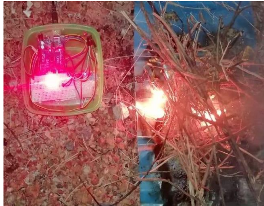
Figure 14. Dry Twig Detection Test
