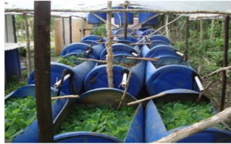
Fig. 2. Monitoring ponds for 5 kinds of local water plant in the phytoremediation process for 29 days .
