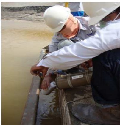
Figure 3. The process of water sampling in acid M2W void.
