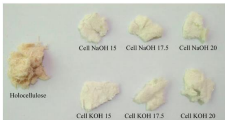
Figure 1. Photograph of holocellulose and \alpha -cellulose from E. dulcis
