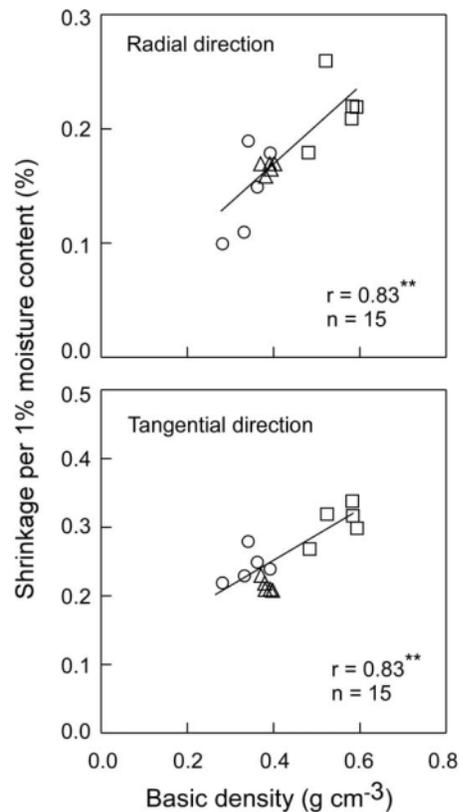
Figure 5.—Relationships between basic density and shrinkage per 1 percent change in moisture content.  $n$  = number of trees;  $r$  = correlation coefficient; \*\* = significant at the 1 percent level.
