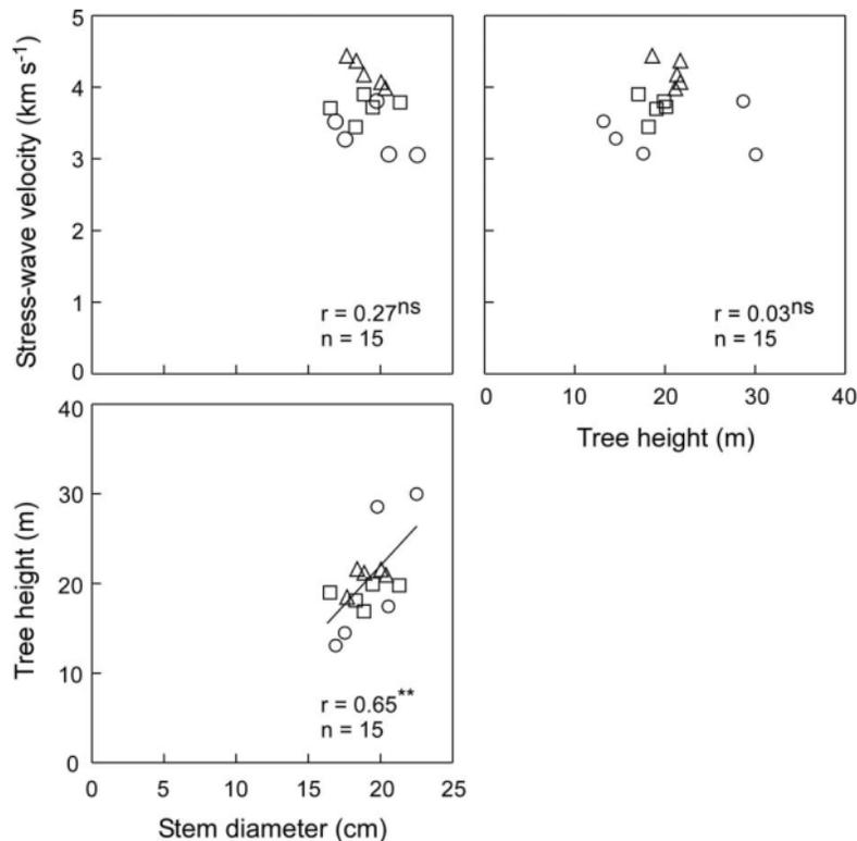
Figure 1.—Relationships between growth characteristics and stress-wave velocity in three species. Circles, squares, and triangles indicate terap, medang, and balik angin, respectively. *n* = number of trees; *r* = correlation coefficient; ns = not significant; \*\* = significant at the 1 percent level.
