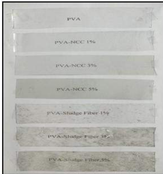
Fig. Transparency of PVA film, composite of PVA and sludge fibers, and cellulose nano composites of PVA reinforced with nanocrystal cellulose
