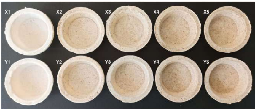
Fig. 6. The physical appearance of starch foams produced by five different concentrations of WHF (0, 5, 10, 15, 20%) with (Y) and without (X) the addition of PVA.
