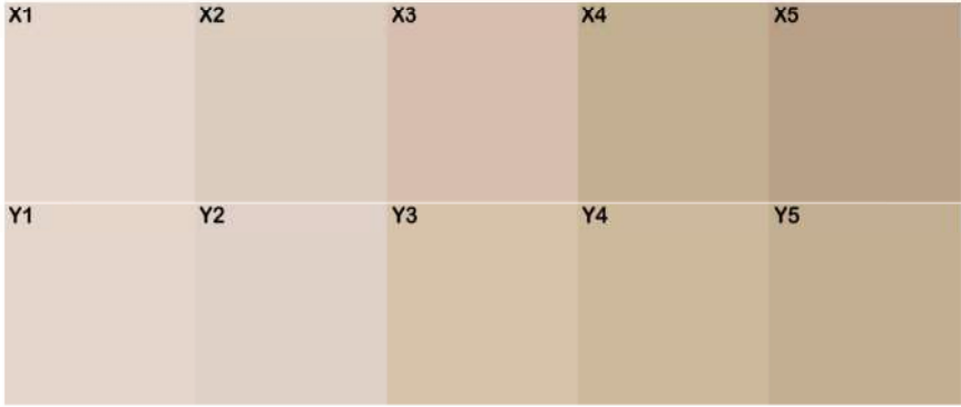
Fig. 7. Color saturation and brightness of starch foams produced by five different concentrations of WHF (0, 5, 10, 15, 20%) with (Y) and without (X) the addition of PVA.
