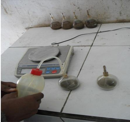
Gambar 1. Analisa Specific Gravity
