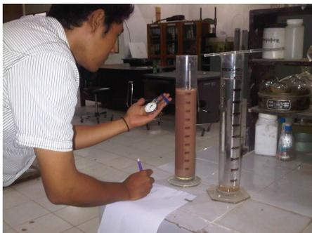
Gambar 7. Hydrometer test
