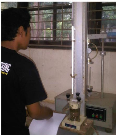
Gambar 9. Permeability test
