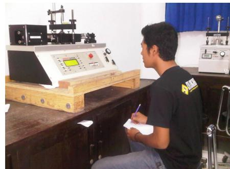
Gambar 8. Direct shear test
