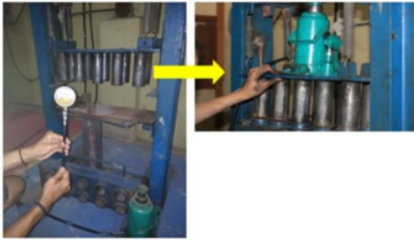
Figure 1. The compaction pressure machine using the hydraulic press machine
