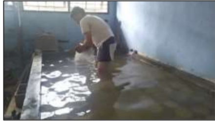
Figure 3. The Treatment of Immersing the Test Object into Water for 7 days
