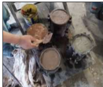
Figure 2. Making a Cylindrical Test Object
