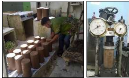
Figure 4. Testing the test object using the Compressive Strength Test tool
