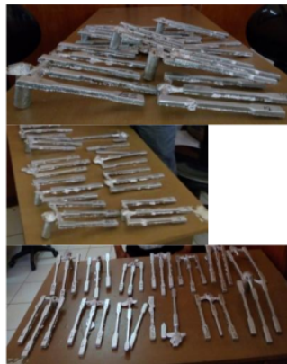
Gambar 4. Hasil (specimen) pengecoran evaporative
