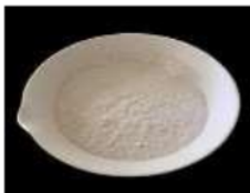
Figure 2. The ash result of Siam Unus Rice Husk
