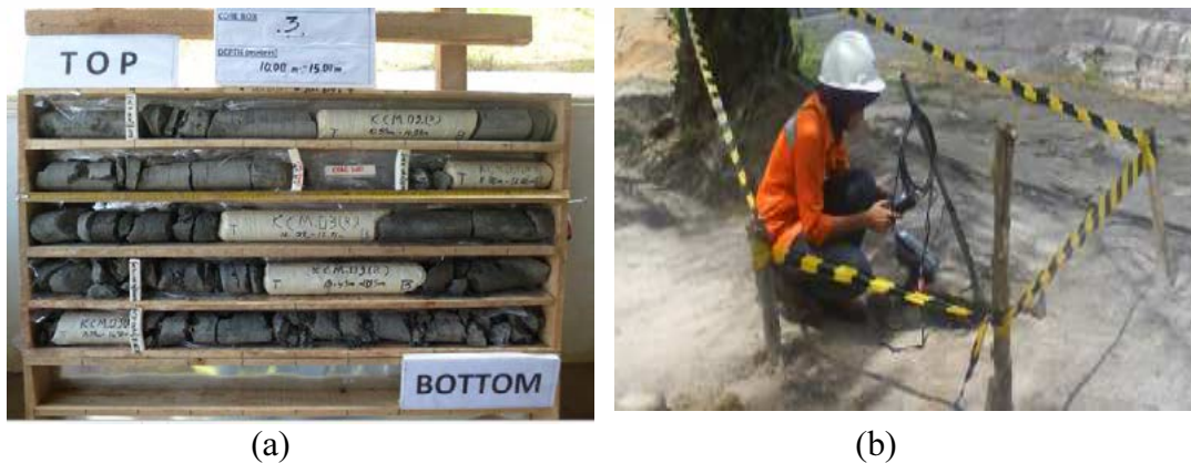
Figure 3. (a) Example of core box, and (b) pore-water pressure measurement
