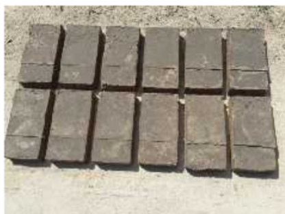
Gambar 7. Proses penjemuran bata
