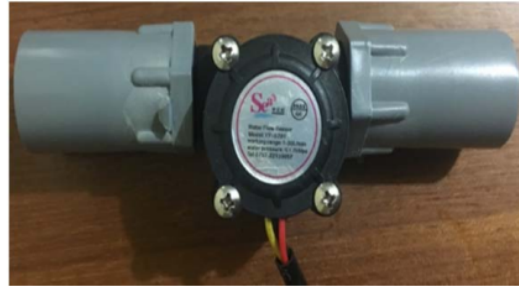
Figure 9. Pipe connected flow meter
