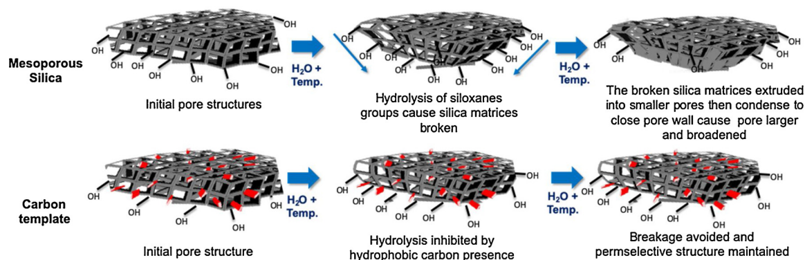
Fig. 10. Schematic of mechanism for stabilization of the carbon template silica pore structure.
